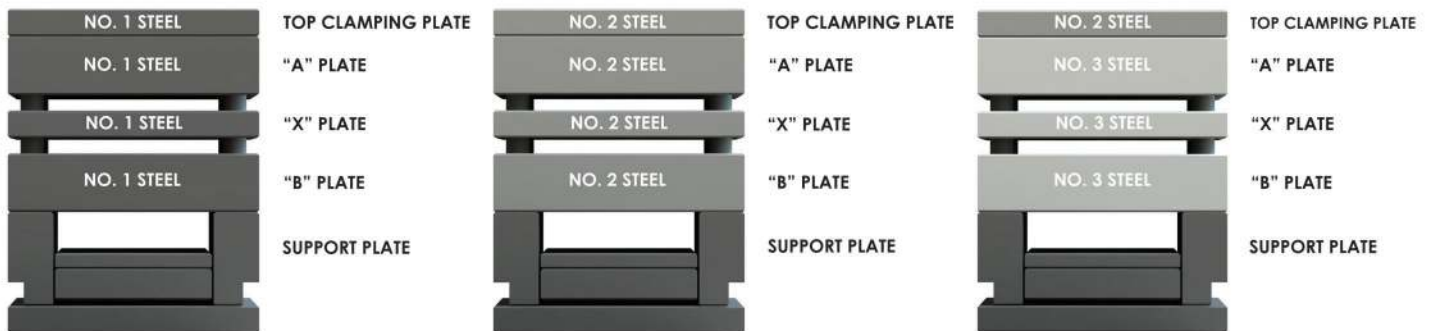
NO.1 STEEL ASSEMBLY
