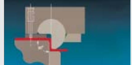
Overbend To 120° in One Stroke
